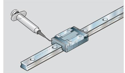
If the **funnel-type lube nipples** on the runner block end faces are preferred, use a **grease gun** instead.
