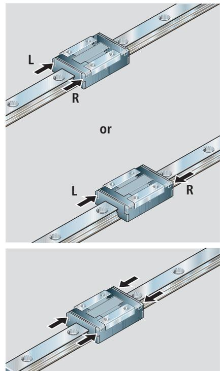
For **short stroke** applications, apply the partial amount per side as given in the table to each end-face lube port.
