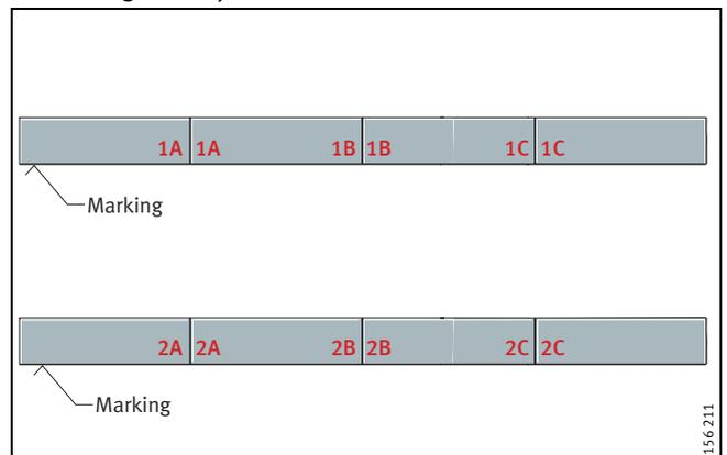
Figure 5 • Marking of multi-piece guideways
