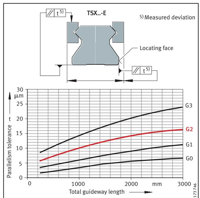
Figure 1 · Accuracy classes and parallelism tolerances of guideways
